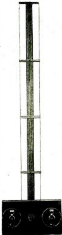
A view of the novel receiver here described with its loop aerial.
