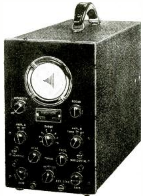
The RCA cathode-ray oscillograph, a typical model of this newest scientific instrument for analyzing conditions in a radio or an electrical circuit.
